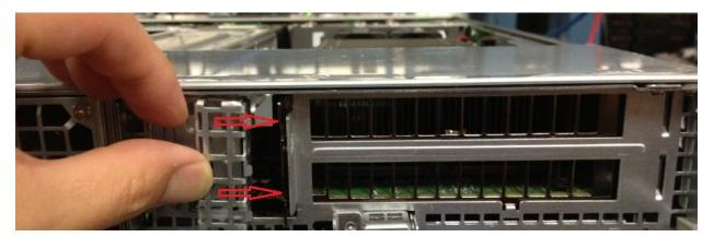
8. Secure the GPU with the 2-mm screw as indicated.
