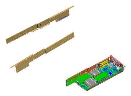
2. Place the adaptor card support plate alongside the power adaptor card so that the holes match up.
