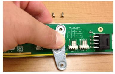
3. Hold the bracket and the sheet metal and, fasten them together with the screws.
