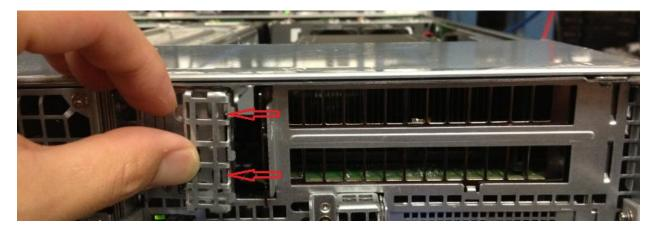
3. Secure the GPU mounting bracket to the GPU itself.
