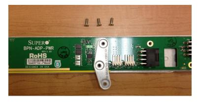
2. Align the holes on the bracket with those on the power adaptor card.
