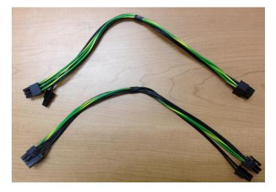
2. Insert the 8-pin connector into JPW1.
