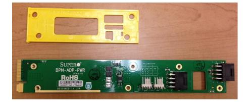
3. Place the plate on the back of the power adaptor card.
