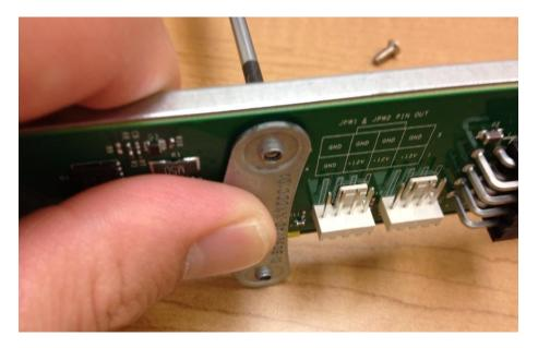
4. Secure the sheet metal with two screws.
