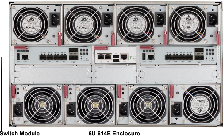
Figure 3-5. 6U 614E Blade Enclosure with Switch Modules Installed
