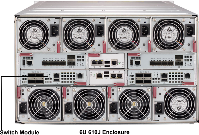
Figure 3-5. 6U 614E Blade Enclosure with Switch Modules Installed
