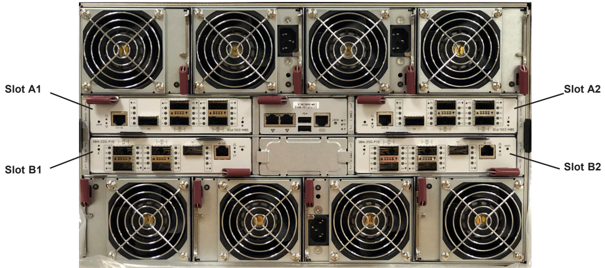
Figure 5. Four Pass-Thru Modules Labeled
