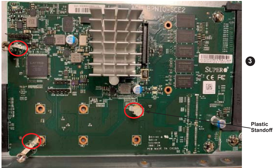
Figure 2-12. Installing the SuperCap Standoffs onto the Bridge Board
