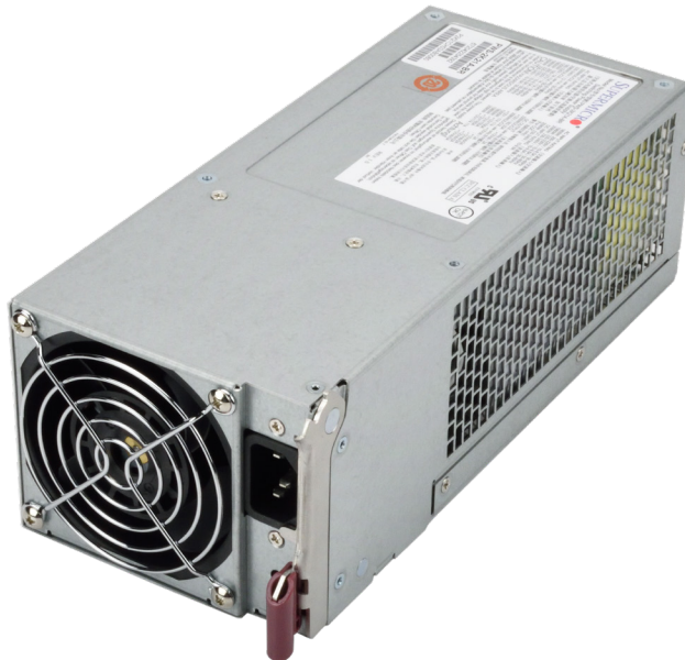
Figure 4-1. Example Power and Fan Module, PWS-2K21A-BR
