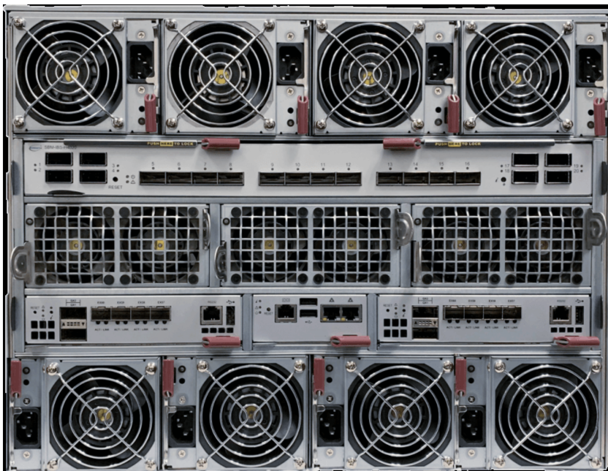
Figure 3-11. Rear Modules Installed
