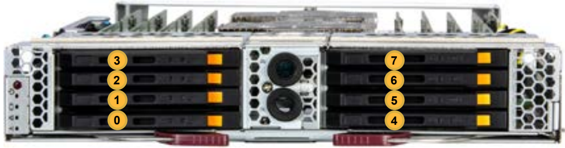
Figure 2-5. Logical Drive Numbers, SBI-621E-1NE38
