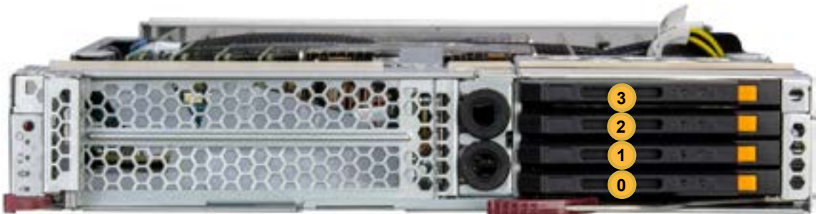
Figure 2-4. Logical Drive Numbers, SBI-621E-1NE34
