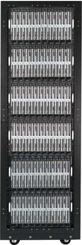
Figure 1-1. Full Rack of Blade Enclosures and Blade Servers
