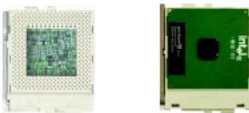
Figure 5-3A. FCPGA Socket: Empty and with Processor Installed
