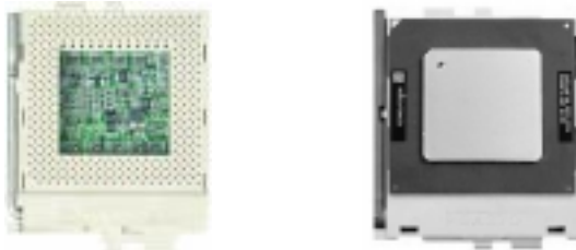
Figure 5-3. FCPGA Socket: Empty and with Processor Installed
