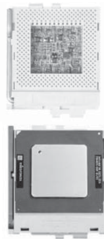
Figure 5-3. FCPGA Socket: Empty and with Processor Installed
