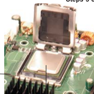
CPU in the CPU socket
