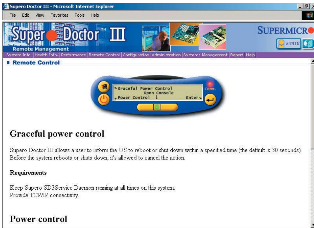
Figure D-3. SuperDoctor: Remote Control Screen
