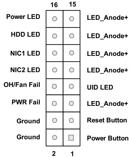
Figure 5-1. Front Control Panel Header Pins (JF1)
