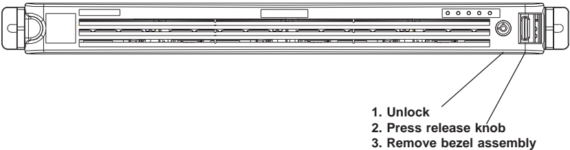
Figure 6-3. Removing the Front Bezel
