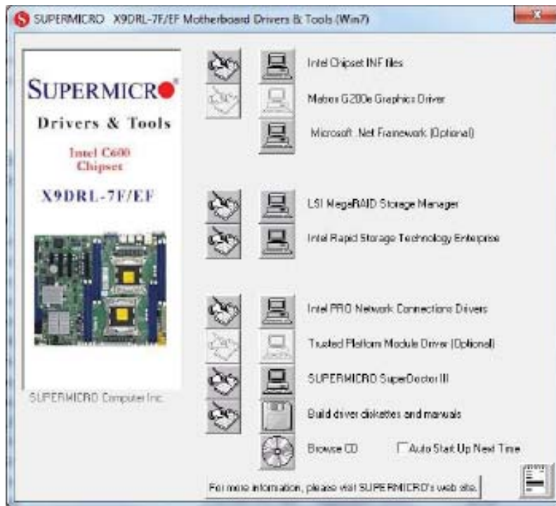
Figure 5-6. Driver/Tool Installation Display Screen
