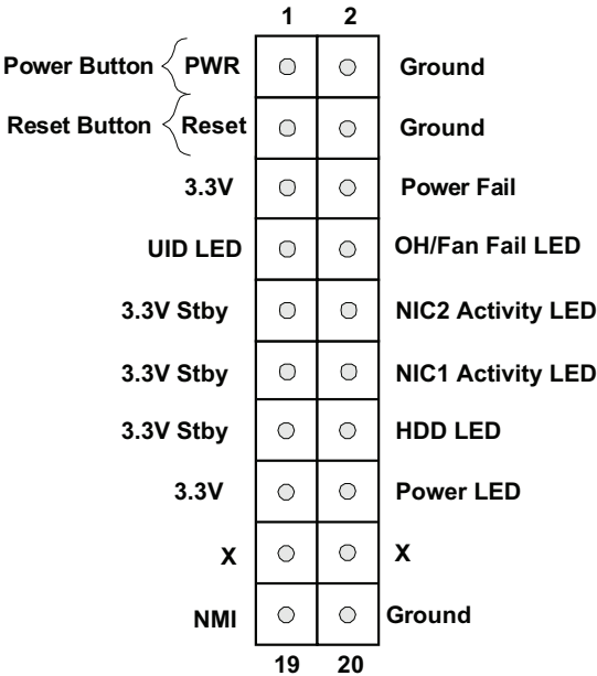
Figure 4-1. JF1: Control Panel Pins
