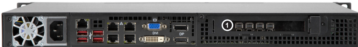
Figure 3-12. Expansion Card Chassis Slots
