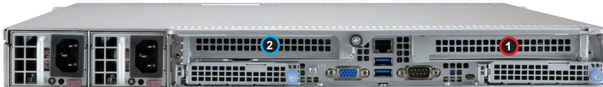
Figure 3-14. Expansion Card Slots in the Chassis
