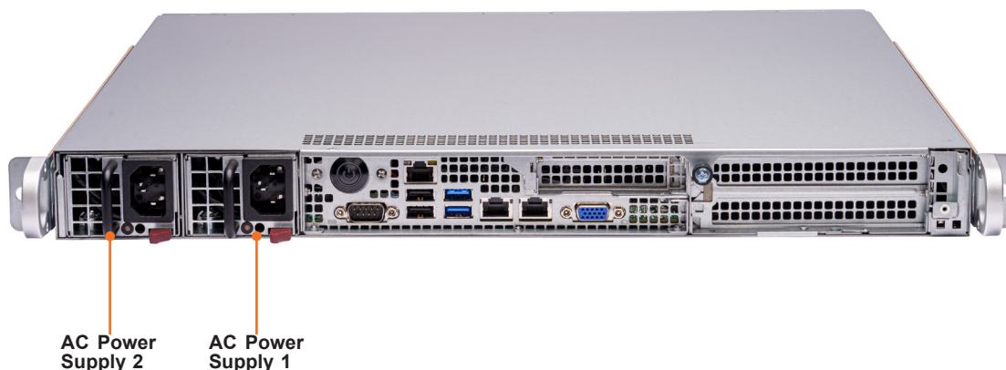
Figure 1-1. Front View of DC and AC Systems
