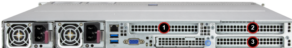
Figure 3-46. Expansion Card Chassis Slots
