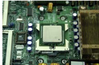
Socket lever in the locking Position
