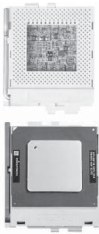
Figure 5-3. FCPGA Socket: Empty and with Processor Installed (Low Power Pentium III shown)
