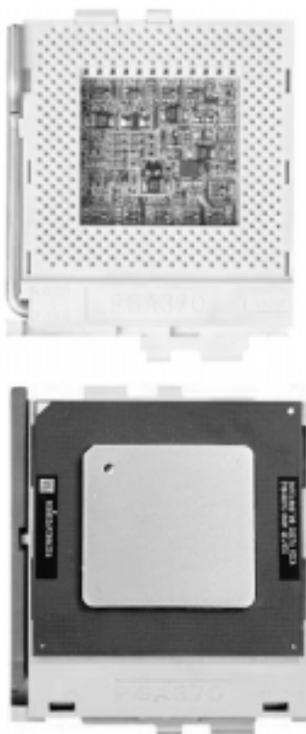
Figure 5-3. FCPGA Socket: Empty and with Processor Installed
