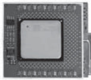
Figure 5-1. PGA Socket: Empty and with Processor Installed
