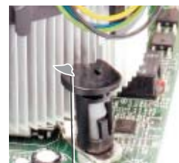
Narrow end of the groove points outward
