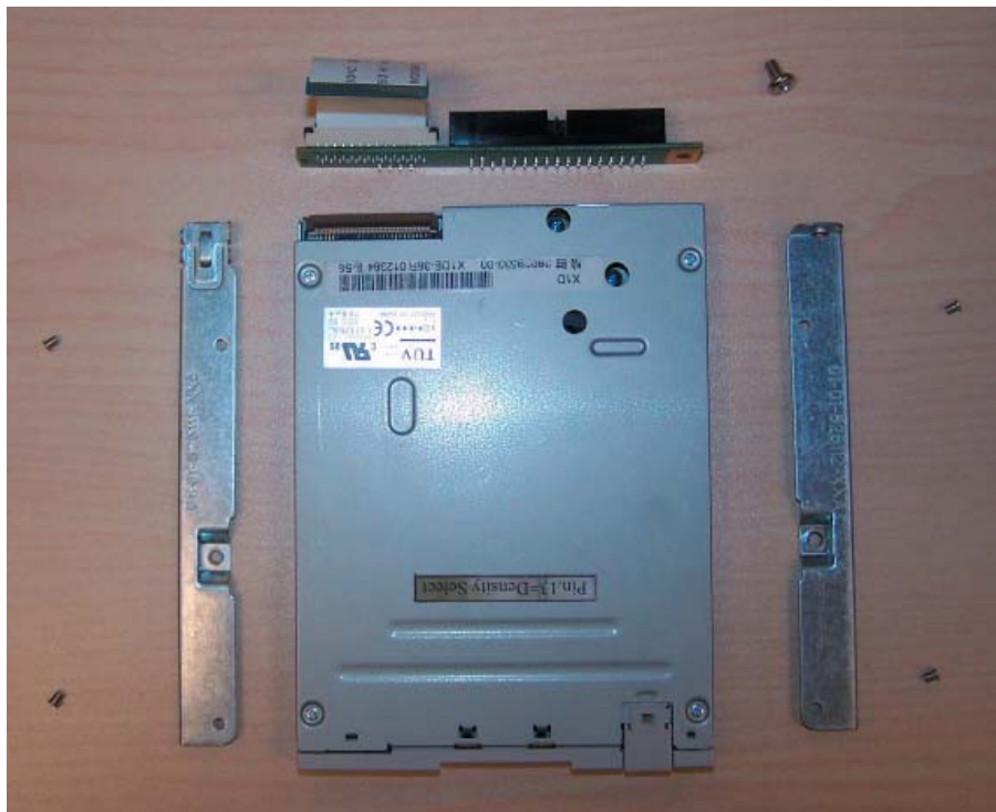
Figure 6-5. Accessory Parts for Slim Floppy Drive
