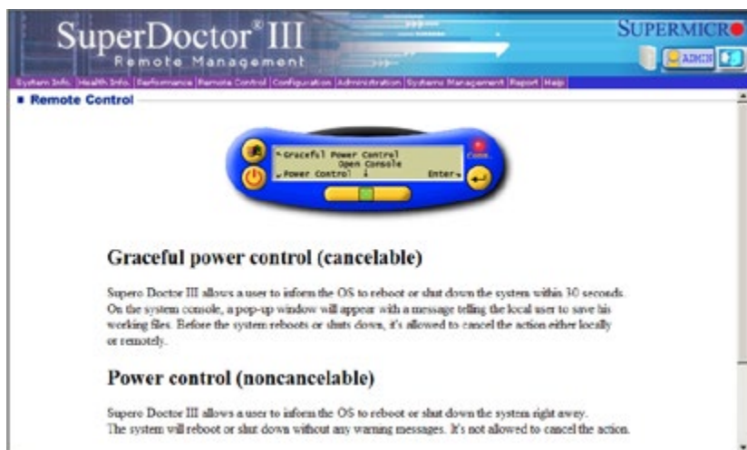
Figure 5-9. Supero Doctor III Interface Display Screen (Remote Control)
