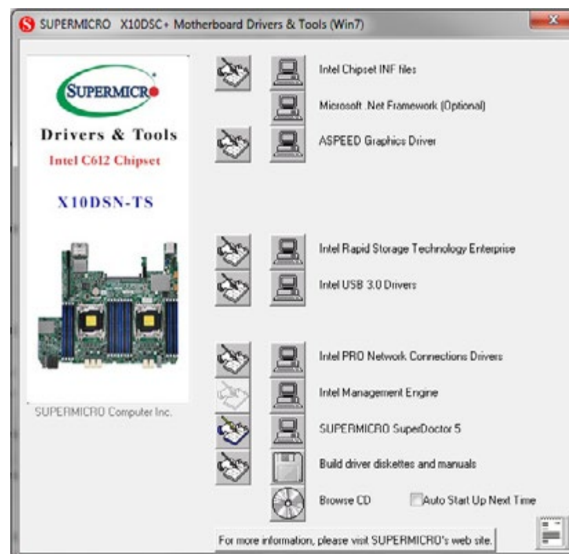
Figure 5-3. Driver/Tool Installation Display Screen
