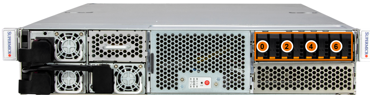
Figure 3-3. Storage Drive Logical Drive Numbers
