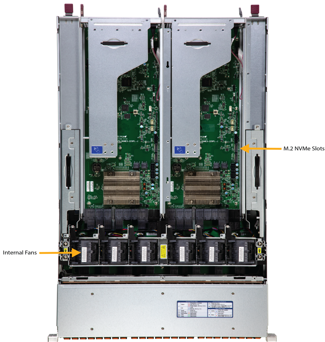
Figure 1-4. SSG-229J-5BU24JBF Main Component Locations
