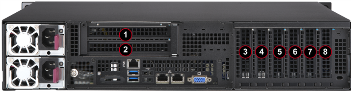
Figure 3-44. Expansion Bracket Locations
