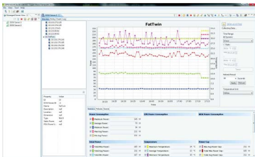
Figure 5-7. SuperDoctor 5 Interface Display Screen (Remote Control)
