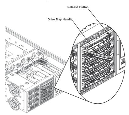
Figure 6-11: Install Hard Drives
