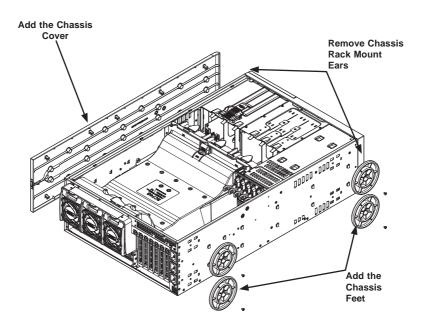
Figure 2-8: Adding the Chassis Feet and Top Cover
