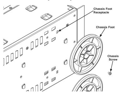
Figure 2-9: Placing Chassis Feet
