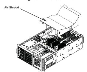
Figure 6-17: Air Shroud in Place
