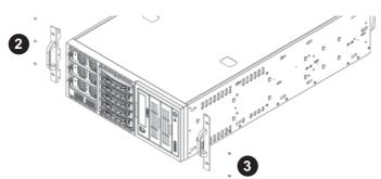
Figure 2-3: Identifying the Chassis Handles
