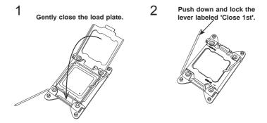
8. Close the load plate with the CPU inside the socket. Lock the lever labeled 'Close 1st' first, then lock the lever labeled 'Open 1st' second. Using your thumb gently push the load levers down to the lever locks.
