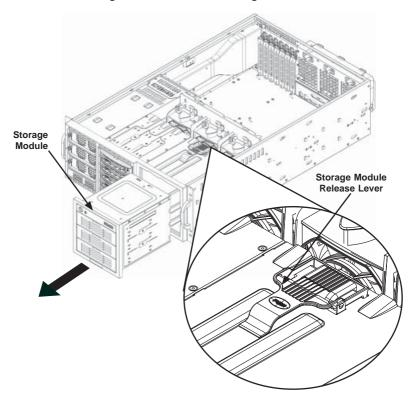
Figure 6-5: Remove the Storage Module
