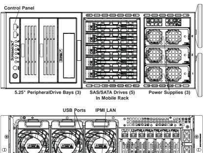
Figure 6-1. Front and Rear Chassis Views
