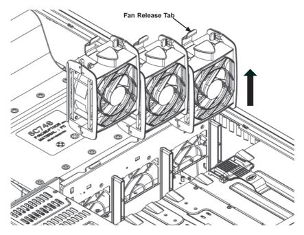
Figure 6-18: Front Chassis Fans
