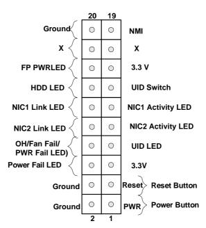
Figure 5-1. Control Panel Header Pins
