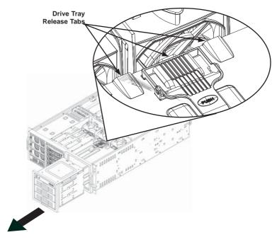
Figure 6-9: Removing the Drive Bay
