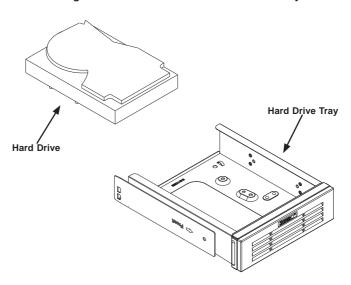
Figure 6-7: Add a Hard Drive to the Drive Tray
