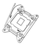
With the lever labeled 'Close 1st' fully retracted, gently push down on the lever labeled 'Open 1st' to open the load plate. Lift the load plate to open it completely.
