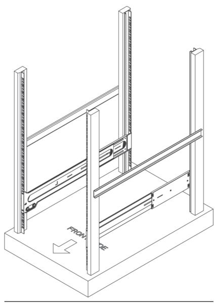
Slide the chassis rails into the rack rails, keeping the pressure even on both sides (you may have to depress the locking tabs when inserting). When the server has been pushed completely into the rack, you should hear the locking tabs "click" (Figure 2-7).
