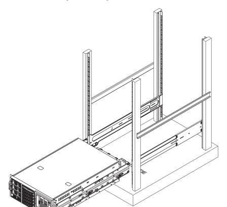
Figure 6-7: Installing the Chassis into a Rack
