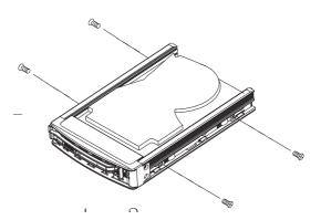
Figure 6-13: Installing the Hard Drive
