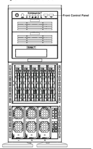
Figure 4-1: Front Control Panel
