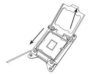
Using your thumb and index finger, hold the CPU on its edges. Align the CPU keys, which are semi-circle cutouts, against the socket keys.
