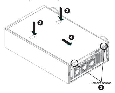
Figure 2-10: Removing the Chassis Cover
