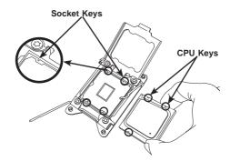
6. Once they are aligned, carefully lower the CPU straight down into the socket. (Do not drop the CPU on the socket. Do not move the CPU horizontally or vertically. Do not rub the CPU against the surface or against any pins of the socket to avoid damaging the CPU or the socket.)
