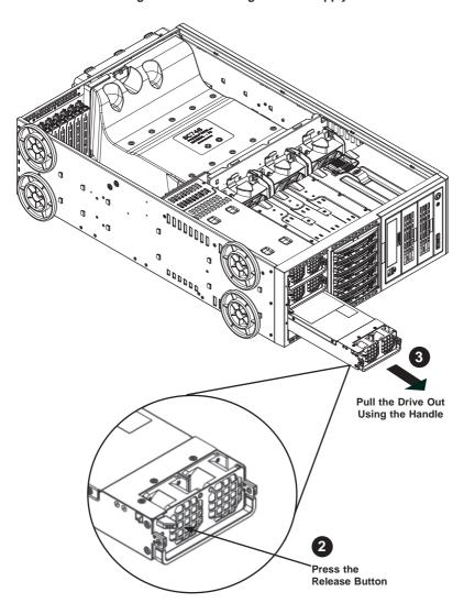
Figure 6-20: Removing a Power Supply
