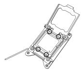
Warning: You can only install the CPU inside the socket in one direction. Make sure that it is properly inserted into the CPU socket before closing the load plate. If it doesn't close properly, do not force it as it may damage your CPU. Instead, open the load plate again to make sure that the CPU is aligned properly.
