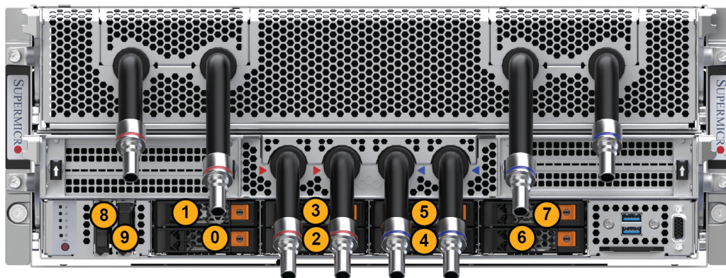
Figure 3-20. Storage Drive Locations
