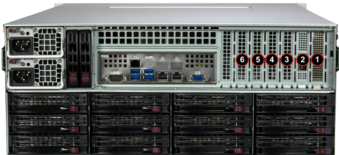
Figure 3-43. SSG-542B-E1CR36H/L PCIe Slots
