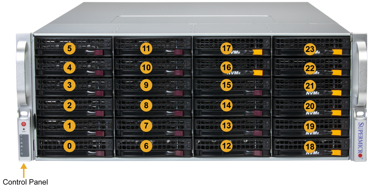
Figure 1-1. SSG-542B-E1CR36H/L Front View
