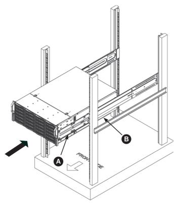
Figure 2-5. Installing the Rack Rails
