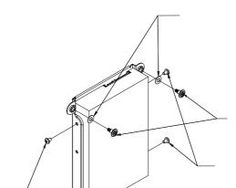
Figure 6-7:Securing the HDD into the HDD Tray
