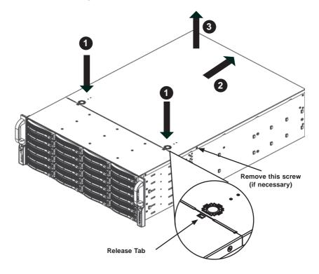
Figure 6-2. Removing the Chassis Cover
