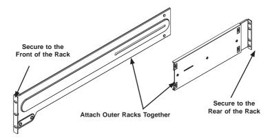
Figure 2-3. Assembling the Outer Rails
