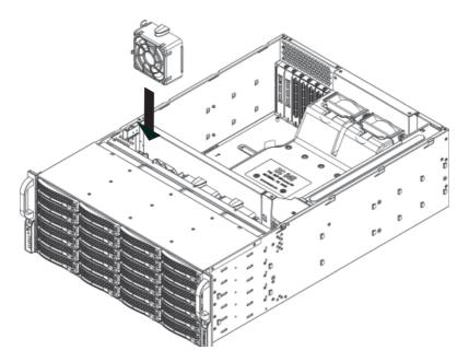
Figure 6-3. Replacing System Cooling Fans
