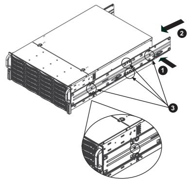
Figure 2-2. Installing the Rails
