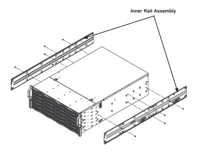
Figure 2-1. Identifying the Rack Rails
