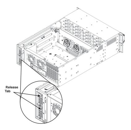
Figure 6-11. Replacing a Power Supply Module
