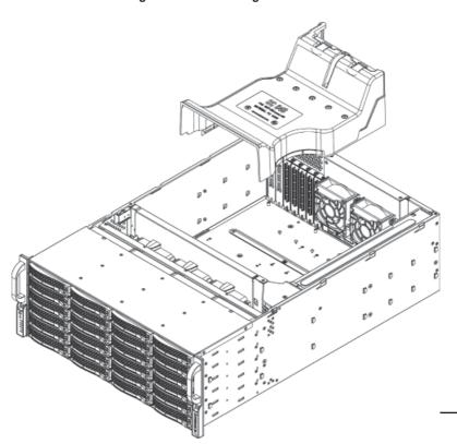
Figure 6-10. Removing the Air Shroud
