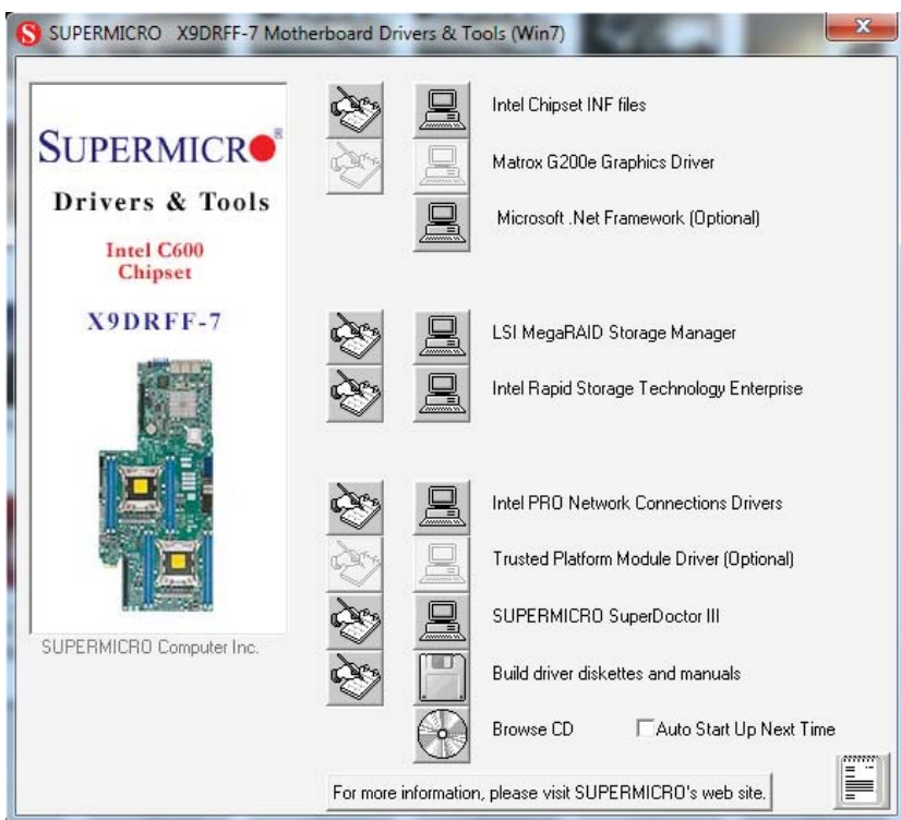
Figure 5-4. Driver/Tool Installation Display Screen
