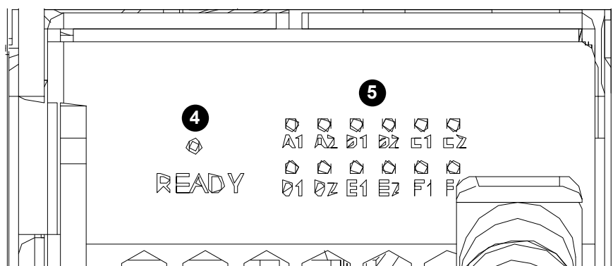
Figure 1-1. CPU Module LED Indicators
