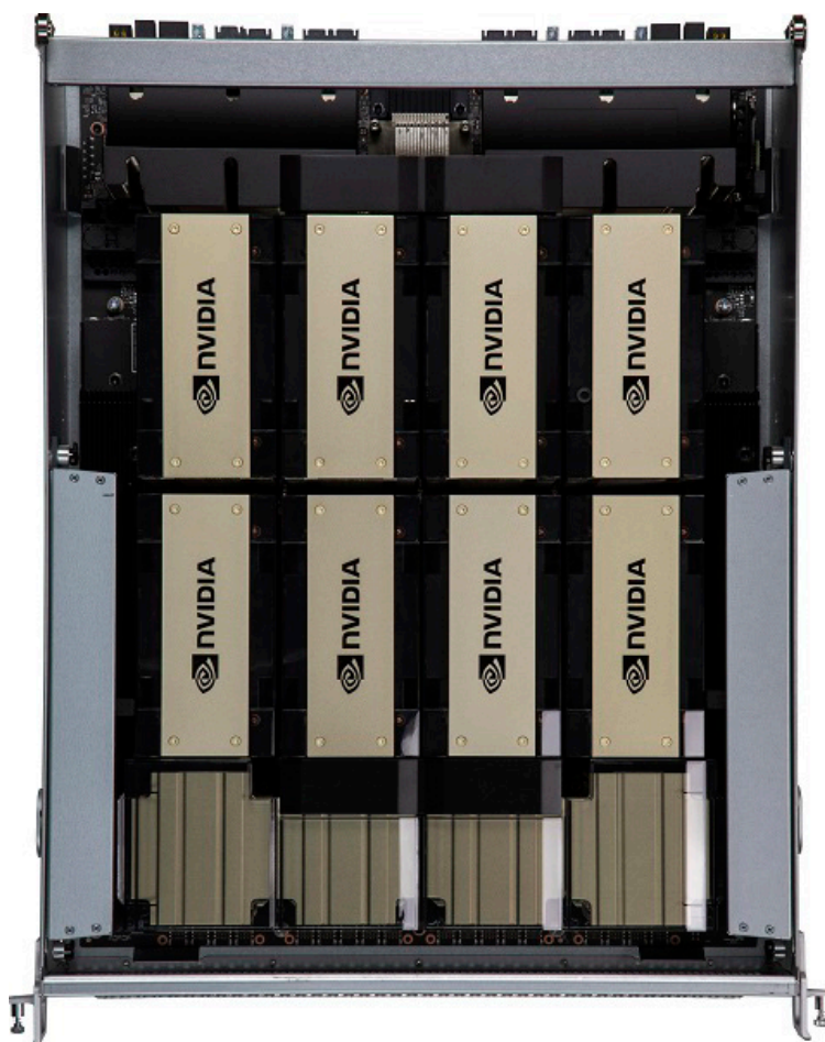
Figure 1-7. Nvidia HGX H100 8-GPU baseboard: Top View
