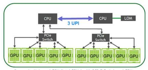
Image 4 - Universal GPU (intel CPUs) with PCI-E Switch and GPUs
