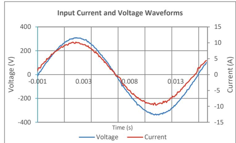
Input AC Current Waveform (ITHD = 1.551%, 50% Load)
