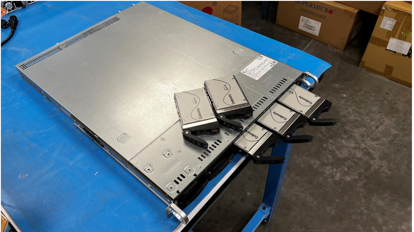
Figure 1- Supermicro 4K Real-time streaming solution (AS-1114S-WN10RT and NETINT Codensity T408 Video Transcoder)
