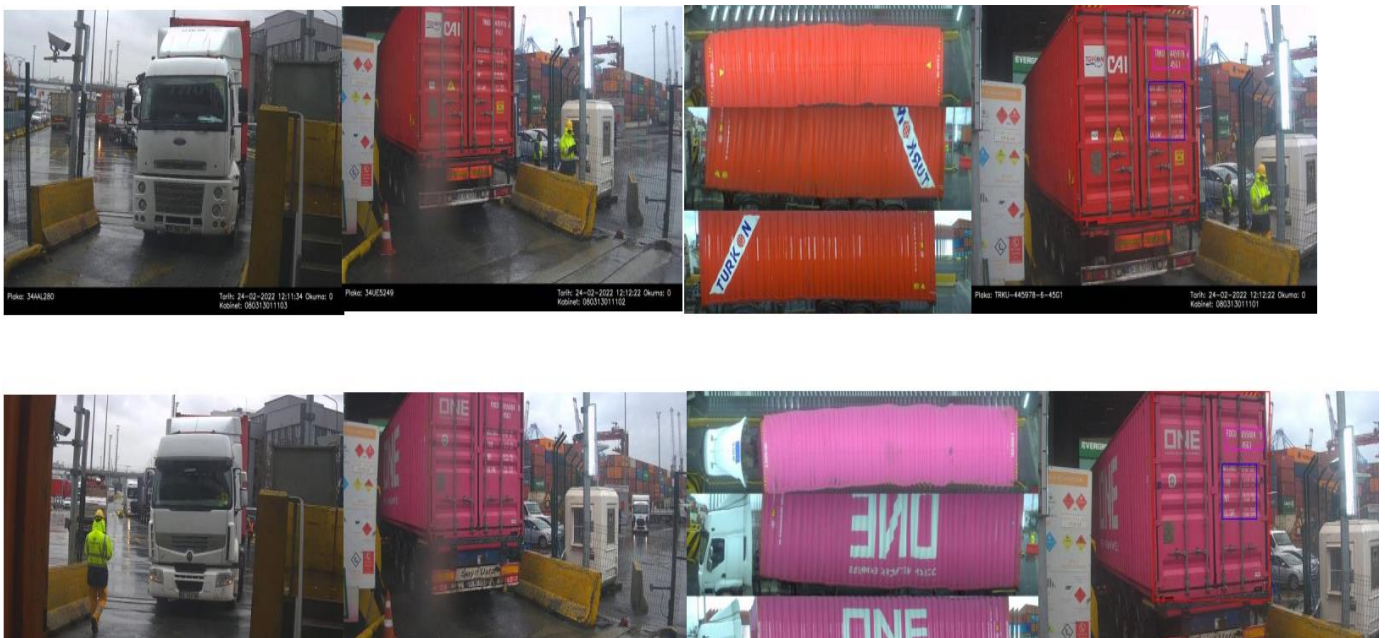
Figure 2 – The ConScan Container and Truck Identification Recognition and Tracking System Output
