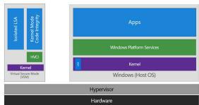
One such security solution example is HVCI, which uses VBS to significantly strengthen code integrity policy enforcement. Kernel mode code integrity checks all kernel mode drivers and binaries before they are started and prevents unsigned drivers or system files from being loaded into system memory.
