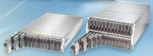
3U/6U MicroBlade 0.05/0.1/0.2U MicroBlade Servers in 3U/6U
