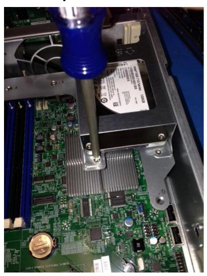
On the bottom of the HDD tray, there were two wedges, you will need to match the wedges into the holes on the tray platform
