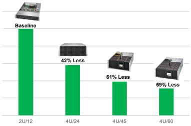
**Figure 1.** Comparative cost per GB Comparison with traditional front-loading servers
