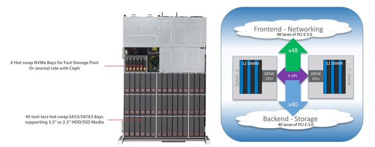
With equivalent I/O bandwidth on both the frontend and backend, users get great performance from the start. This also enables advanced users the ability to configure the hardware and optimize their software to meet their application requirements.
