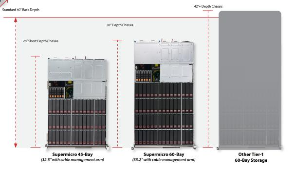
Figure 6. An illustration of server depths in a data center setting
