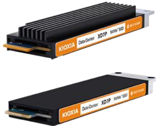
Image 2 - E1.S – 15mm with cooling fins and 9.5 without cooling fins
